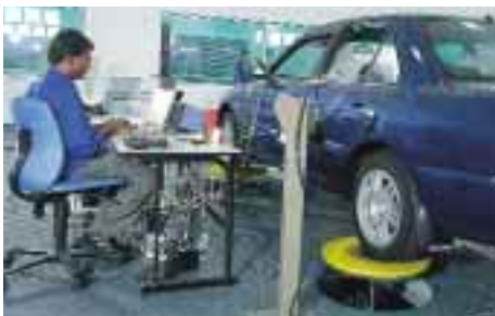
Utilizing the 4 Poster Road Simulator to analyse the car's reaction on different road surfaces.
