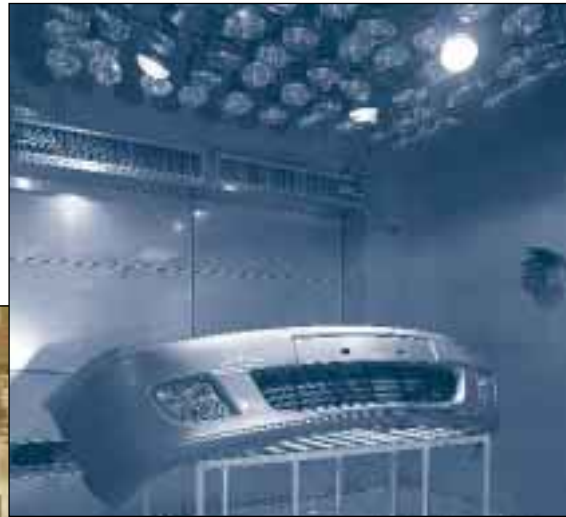
Weather meter test to simulate weather resistant effect on exterior parts.
