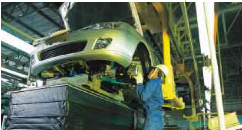
Engine installation at WAJA assembly line.
